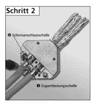
Guide the cable into the lower housing section.
