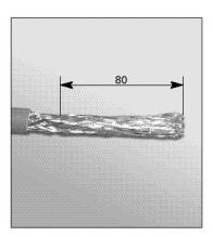
Cut cable shield to length by ...
