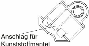
Shorten and prepare cable. For plastered-in cables, ensure a minimum length of approx. 140 mm up to wall!
