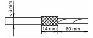
With thinner cables (under 6 mm dia.), braiding is pushed back over sheath and shortened to 14 mm
