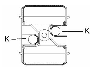
For cables with a diameter over 10 mm, we recommend opening the cable entries (K) in the cover at the marked points with a pair of diagonal cutters after laying on the wires
