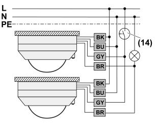
Figure 10: Connection diagram, parallel circuit for expanding the detection field
